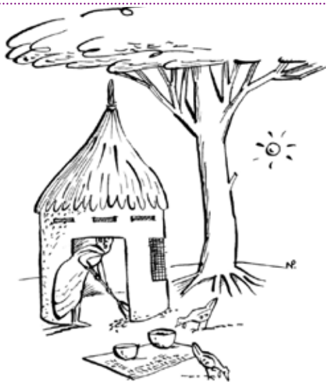
Figure 6: A well-constructed chicken house is placed in the shade, has a high roof and windows with wire mesh, providing good ventilation but preventing entrance of snakes and rats. The door is facing south or north to avoid direct sun. The door is big enough for a person to enter to clean the house frequently (source Riise et al 2004)
