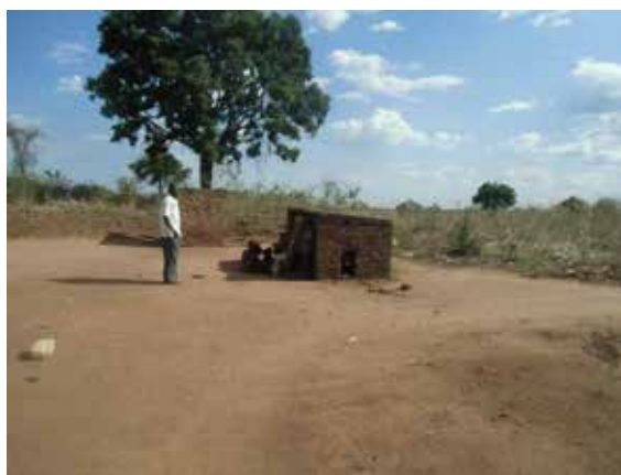
Figure 5: A badly constructed chicken house is placed in the sun with a low flat roof and no windows making it very hot and not well ventilated. It has a small door, which makes it difficult to access and clean it (source Riise et al 2004). On the right is an example of the house in Yumbe district.
